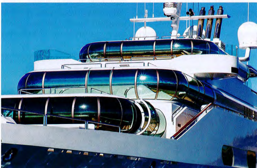
"Enigma": this Martin Francis design, delivered in 1991 named "Eco", features a spectacular superstructure with spherically curved glass panes made by Flachglas.
