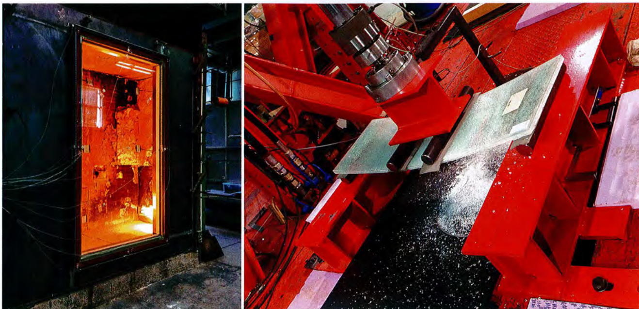
Material testing: glass suppliers have to prove how strong, dense or fireproof their panes are. The flexural strength test (r.) provides information about bend strength, while fire-retardant glass (l.) has to withstand temperatures of up to 1000 degrees Celsius.
