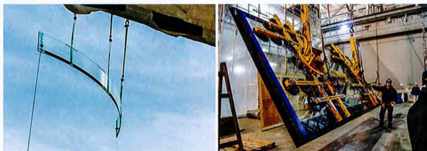
Tricky handling: GL Yachtverglasung delivered the world's longest curved pane of glass (15 metres) for the yacht, "A" (l.). Four-tonne glass panes (r.) are routinely moved around.
