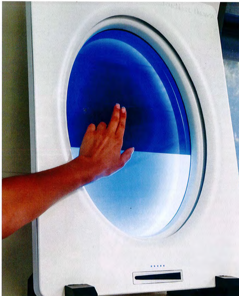
"Nuance": Vision Systems developed an electrically dimmable solution, which is already used on aircraft and which is now set to conquer the yacht market.
