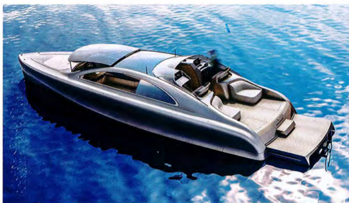
"Arrow 460 Granturismo": Vision Systems of France supplies side windows for this 14-metre Silver Arrows Marine day cruiser, which can be lowered using an electric switch. The large roof window sports an electric dimmer function and can also be raised.
