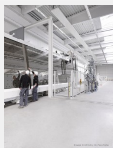
sedak’s new 145-meter-long production line is fully automated to produce insulating glass units up to 3.2 meters by 15 meters. (photo: Rene Muller)
