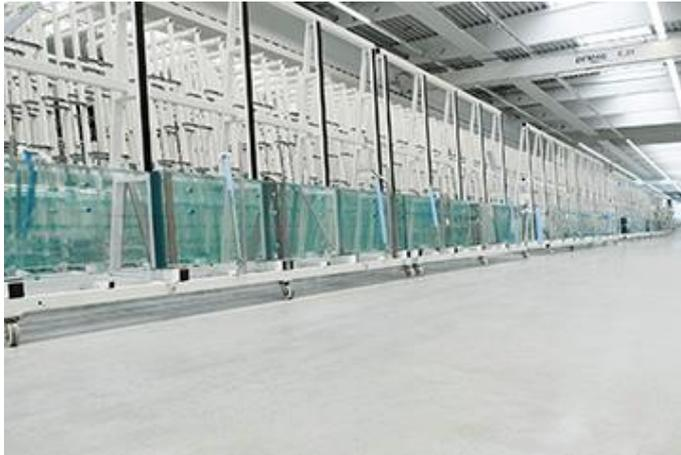
Glass fins, available from sedak in lengths of up to 20 metres, are supporting elements of glass façades. A glass fin that is 20 metres long and weighs 1.5 tonnes is being presented by sedak at BAU (hall C3, stand 100)
