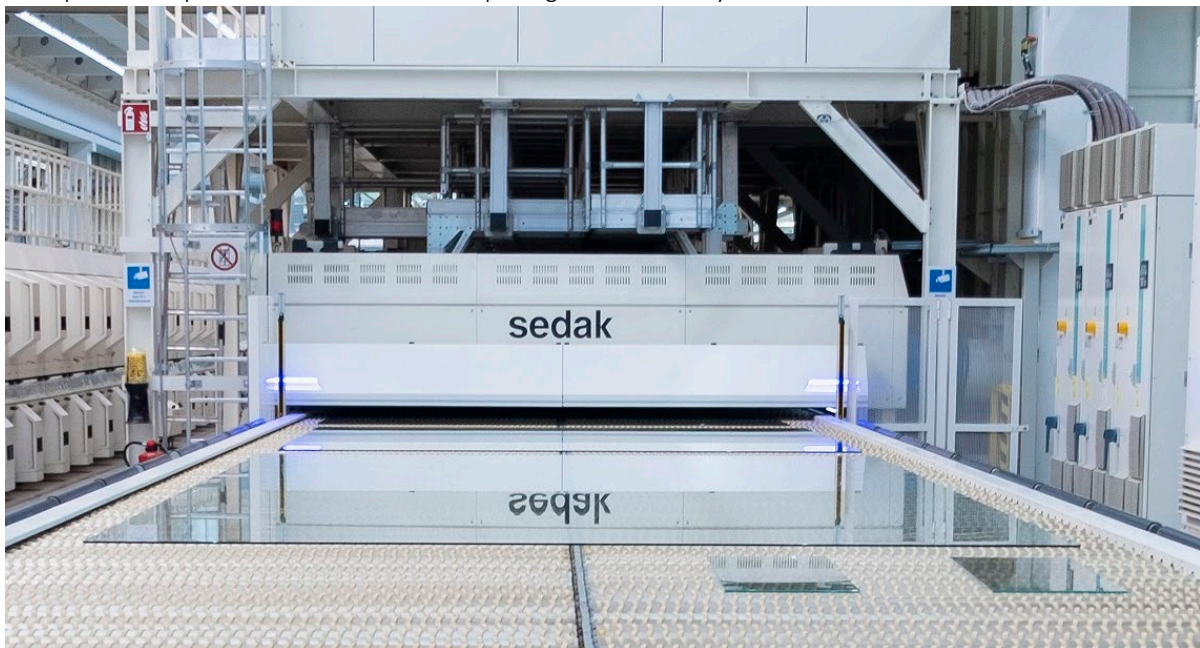
This sedak scanner inspects and documents all glasses that are tempered on our furnace.
