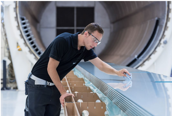
Figure 2: The vacuum process ensures process reliability for thicker glass and especially for multiple laminates.
