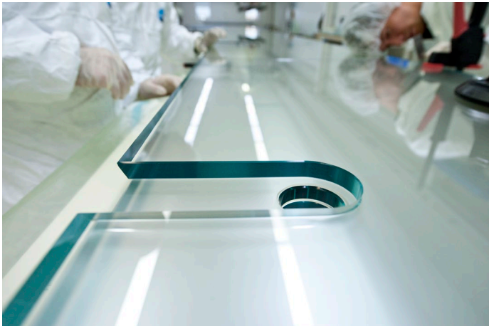
Figure 1: Under cleanroom conditions, sedak glass is layered using interlayers to make a single package.
