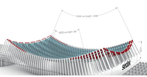
**sedak**'s furnaces can bend glass into double-curved geometries up to 3.6 m x 6.5 m and cylindrical shapes up to 3.6m x 18m, with various radii.
